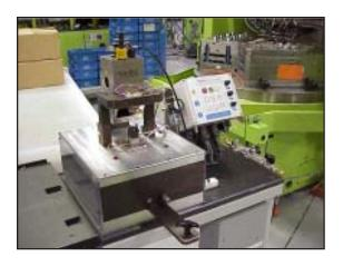
The customer's machine shop produced the custom mounting brackets for the Kortho Print Heads and Controls. The results are extremely clean installations in the close quarters of the inspection systems.
