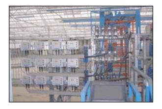
A producer of seedlings uses an automated processing system to pick and sort inventory for customers orders. When the various trays of seedlings are picked from the greenhouses, a bar code containing customer order information is applied to each tray. All of the trays are automatically routed to one of three conveyors for transport to the area where the trays are palletized for shipment.
