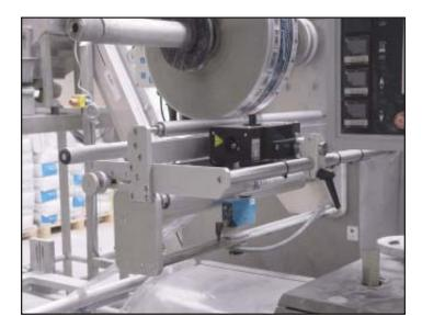
A candy manufacturer uses a Klockner-Hansel horizontal flow wrapper to individually pack large gum balls in a colored plastic film. The Kortho Hot Quick Coder is used to apply 3 lines of 2.5mm code to the film including product code, manufacturing date and expiration date.
