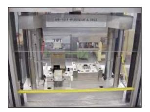
A manufacturer of precision electronic components required a marking system to apply an acceptance spot mark on assemblies after passing continuity testing. Liquid ink marking systems were not an attractive option due to the potential for possible contamination of the sensitive test equipment. The Kortho Hot Ink rolls provide an extremely clean and reliable marking alternative. Kortho HQC Systems were installed on each of three inspection systems in this facility.
